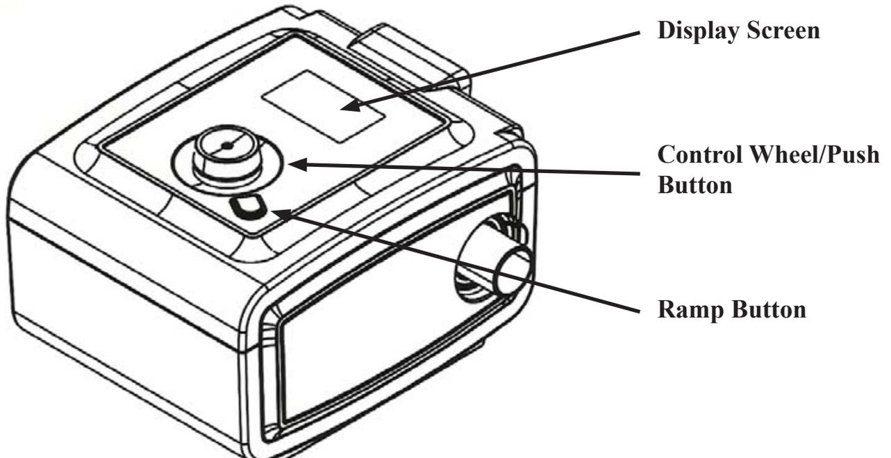
The Display Screen must have the Therapy mode selected for the CPAP/BIPAP machine to turn on.
